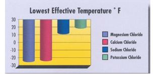
Whether blended with other de-icing materials or applied as 100% magnesium chloride hexahydrate crystals, MeltDown Absolute Zero is the most effective de-icer at low temperatures when safety and environmental impact is considered.
